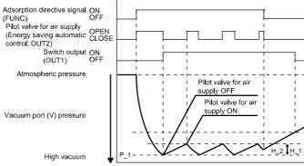
: When turning off the supply pilot valve with a vacuum pressure which is higher than the set value (P\_1), and other setting methods, refer to the operation manual which can be obtained from the SMC website (URL http://www.smcworld.com).
